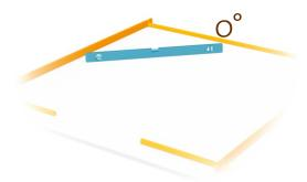
MAKE SURE THAT THE BOTTOM LOGS ARE INSTALLED ON A LEVEL SURFACE. CHECKING ALL DIRECTIONS, INCLUDING CORNER TO CORNER. 2%
